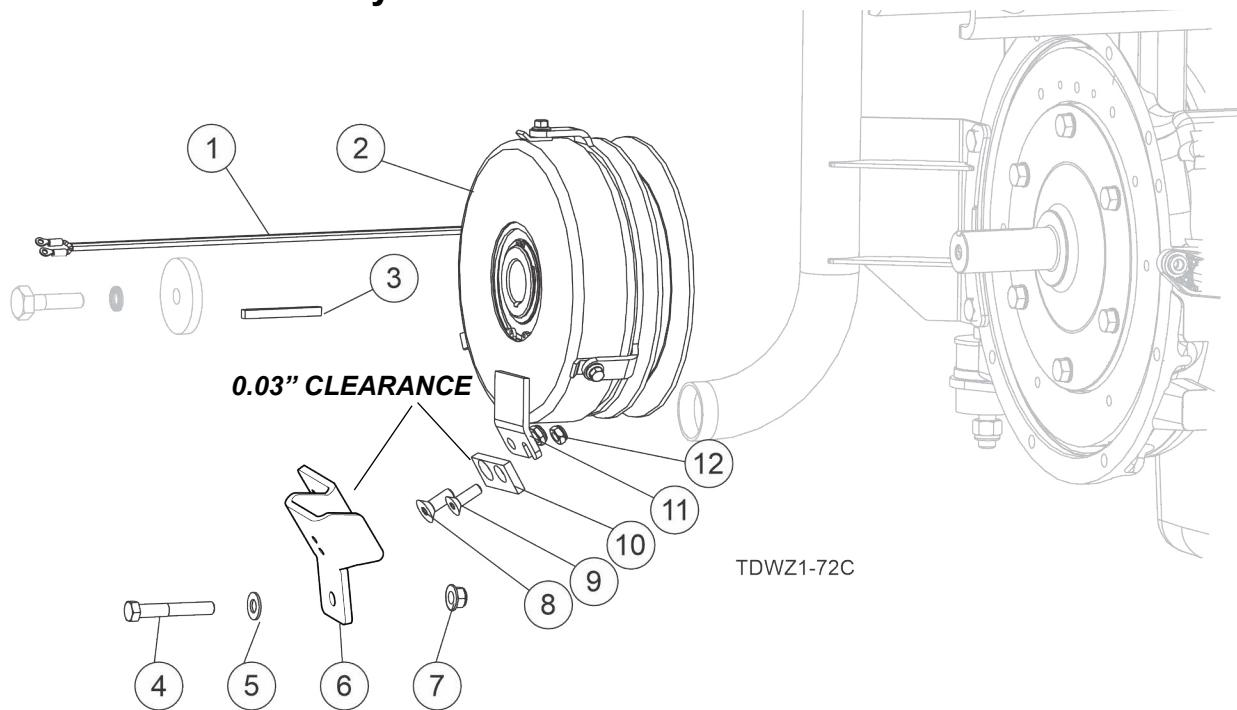
**ENSURE 0.030" CLEARANCE BETWEEN THE CLUTCH STOP BRACKET (6) AND PAD (13)**
